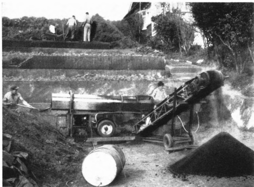
Fig. 1.—Flash-Flame Soil Sterilizer being used at Messrs. Carew's Nurseries, Erson Avenue, Onehunga, Auckland. Note steam rising from the stock pile being delivered by conveyor. (See page 220). (S. A. Rumsay)
